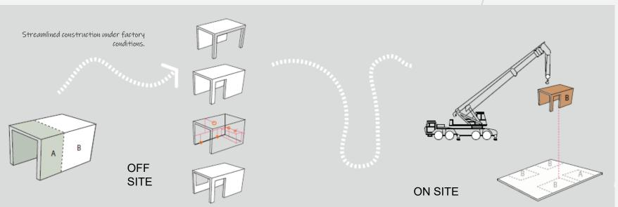
Two different sized pre-fabricated concrete modules for the basic building blocks for a project design.
